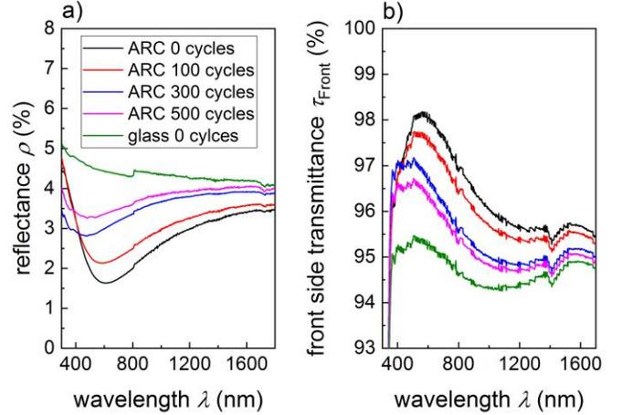
Fig. 5. a) Spectral reflectance with back side absorber structure indicating the front surface intensity reflection factor  $R_{\text{FS}}$ . b) Spectral transmittance of the front side calculated from the reflectance measurements via LoEC approach (eq. 5).
