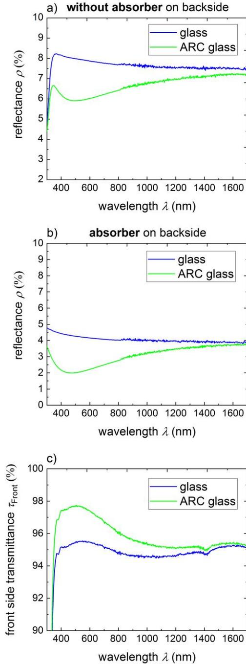
Fig. 3. Spectral reflectance of the samples without (a) and with (b) backside absorber that is suppressing the backside reflection. The hemispherical spectral transmittance of the glass front side  $\tau_{\text{Front}}$  (c) is calculated from the reflectance without backside reflection and the bulk absorption determined on uncoated glass samples.
