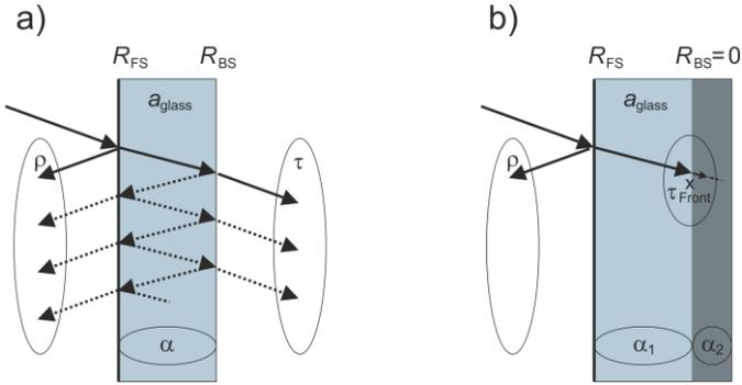
Fig. 1. Optical conditions of the incoming light intensity of glass in air (a) and a glass with index matching at the back side (b) corresponding to the sample systems for greenhouse and PV applications, respectively.
