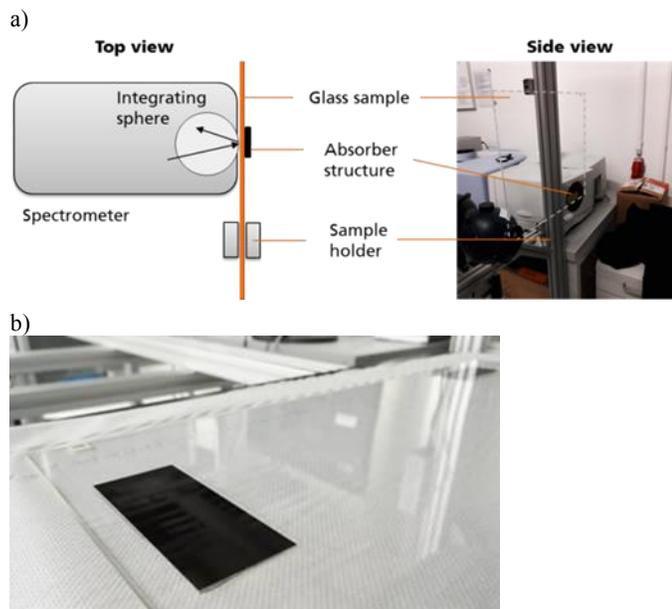
Fig. 2. a) Reflectance/transmittance measurement setup for large samples schematically in top view (left) and as experimental setup in side view (right). b) Detail view of a glass pane with the broad band absorber applied to the back side.
